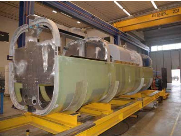
A DS-8 SDV under construction in Romania. (Photo: DRASS)
